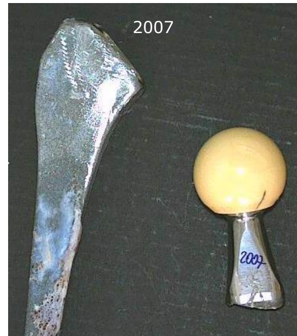
Implant fracture: neck
